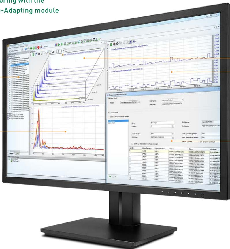
Real time visualization of the spectra as an individual spectrum, waterfall or contour view
