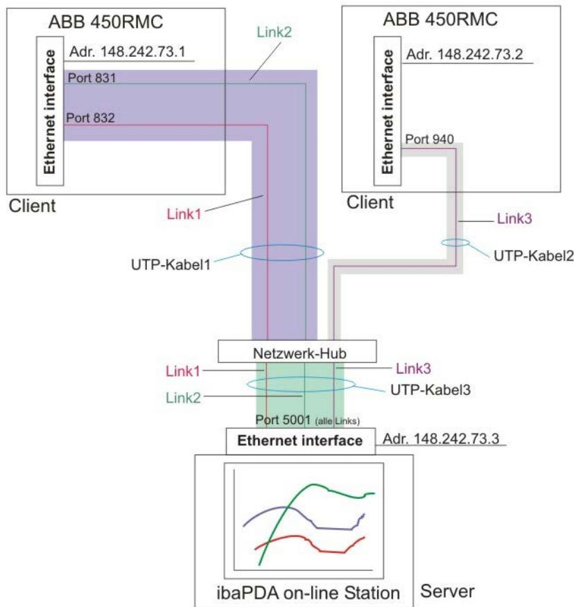
Regarding figure *Communication Principle ibaPDA - ABB AC450RMC 3* please note that two ABB AC450 controller act as clients, whereas every controller has its own Ethernet module which is connected to the network with one cable each. There is another cable which connects *ibaPDA* with the hub (the cables are displayed here in different thickness and colour). The network has three communication partner with unique IP address each.
