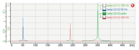
The legend has a drag & drop function. This way, a spectrum can be laid upon different value axes. While dragging the spectrum, an arrow appears in the value axis tree pointing to the tree that will contain the spectrum when it is dropped. If a spectrum is not dropped inside a legend row, the spectrum will be laid upon a new axis.
