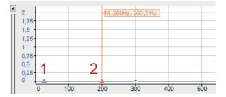
The example above shows a collapsed marker (1) and a normal marker (2).
