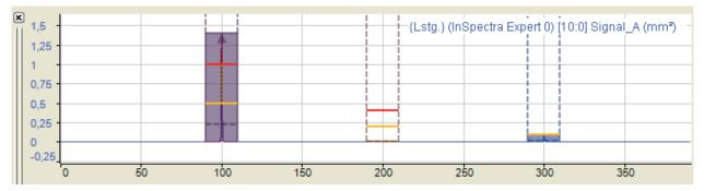
In the figure above the display shows three different frequency bands and at least a part of the spectral graphs from the main window. You can add additional graphs by dragging and dropping them from the main window or from the signal tree via drag & drop. The displays are linked so that all graphs in the small spectral display can also be seen in the main window.
