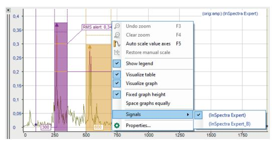
If there are several spectra in the display, individual display properties can be assigned to every spectrum.
