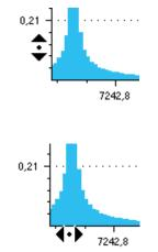
You can also use the mouse wheel to zoom in or out around the center of the axis. Note that you can never move outside the scale extremes of an axis.
