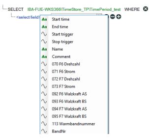
Depending on the selected field (numeric or text field), clicking on the green equals symbol displays a list of operators. Select the required operator.
