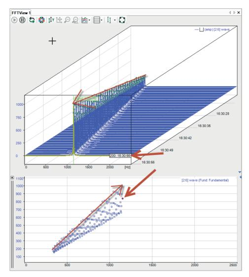
This display does not have its own interactive marker. When you hold down the <M> key, the mouse moves over the points and the corresponding values (X, Y, and plane) are displayed in a pop-up.
