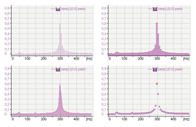
The option *Improve isometric visibility* is used to make spectra opaque. This makes some effects in the waterfall view more visible.
