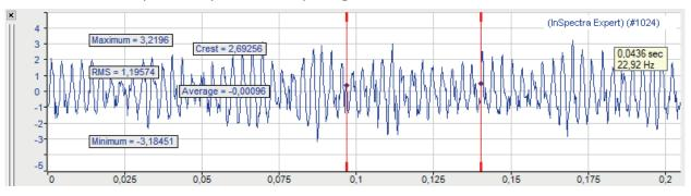
If the averaging function was enabled in the calculation settings of the profile, then the display shows the time signal of the last internal FFT calculation. The displays of the FFT results in the main window and frequency range, however, are also based on prior values of the input signal.
