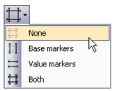
If a marker type is active, it is displayed on the chart and can be moved. More information on markers is displayed between the markers or in the signal table below the chart.
