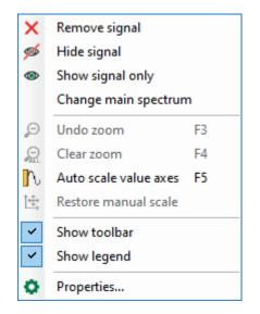
Clicking on "Remove signal" removes the corresponding signal. Clicking on "Hide signal" hides the signal and shows the signal name transparently. The signal is only temporarily hidden and can always be displayed again. By clicking on "Show signal only" in the context menu, only the selected spectrum remains in the display and all other spectra are hidden. Clicking on "Change main spectrum" makes the selected spectrum the main spectrum.
