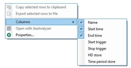
In the upper section of the context menu, you can select the standard columns, and in the lower section the columns for the info fields. The info field columns that appear in the context menu can be configured in the properties of the time periods table, see next section.
