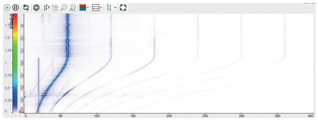
The color scheme can be configured in the properties of the value axis. Both pre-defined schemes can be selected here and customized color schemes can be created.
