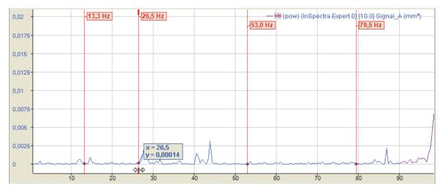
The above figure shows an interactive marker with 1 harmonic component below and 2 harmonic components above the marker frequency of 26.5 Hz.
