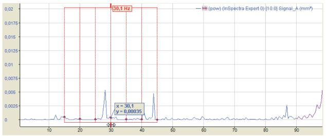
The above figure shows an interactive marker with 3 sidebands and offset of 3 Hz each.
