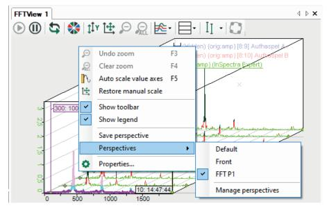
Scales are always displayed at the side of the chart not overlapping with the perspective flow direction. Several spectra can have different sample rates or bin values and thus the clock in which the FFT results are available may vary. That is why it is pre-set that every spectrum moves on the Z-axis at its own pace.
