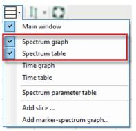
Graphical display and data table form one group, as the table always provides the data matching the spectrum in the graph. However, the graph and table can be individually displayed or hidden.
